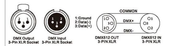
For installations where the DMX cable has to run a long distance or is in an electrically noisy environment, such as in a discotheque, it is recommended to use a DMX terminator. This helps in preventing corruption of the digital control signal by electrical noise. The DMX
