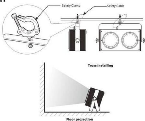
Regardless of the rigging option you choose for your LAB-902A1(WW)B always be sure to secure your fixture with a safety cable. The fixture provides a built-in rigging point for a safety cable on the hanging bracket as illustrated above. Be sure to only use the designated rigging point for the safety cable and never secure a safety cable to a carrying handle.
