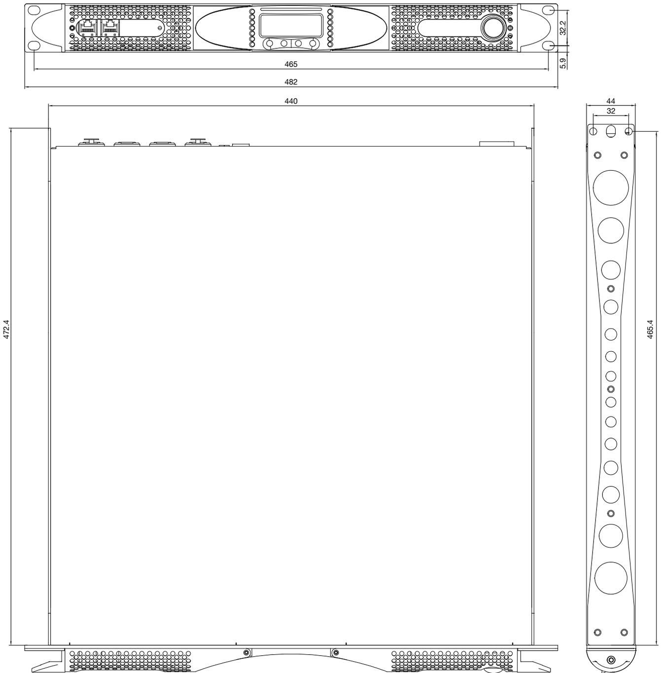
FIGURE 3: K6, K8, K10 and K20 mechanical drawings.
