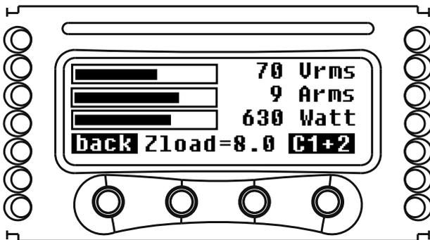
FIGURE 47: Display: Output meters.
