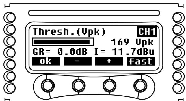
FIGURE 31: Peak limiter: threshold voltage and gain reduction.
