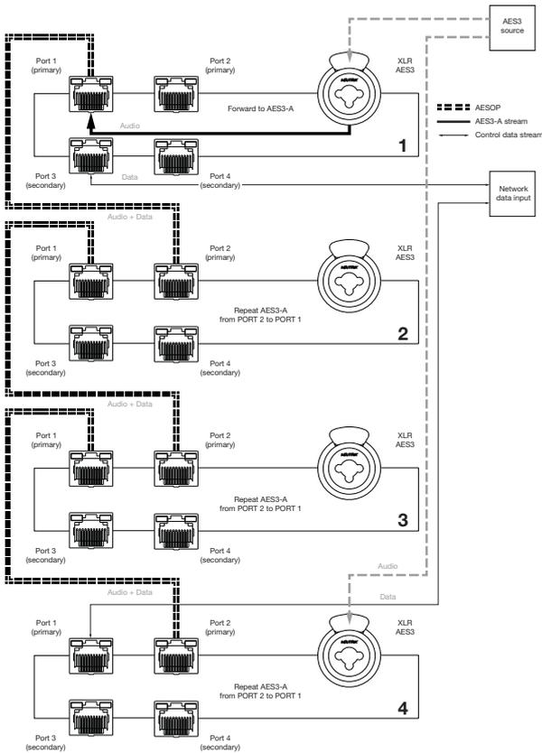
FIGURE 44: Daisy chain with AES3 and Ethernet redundancy - four port models.
