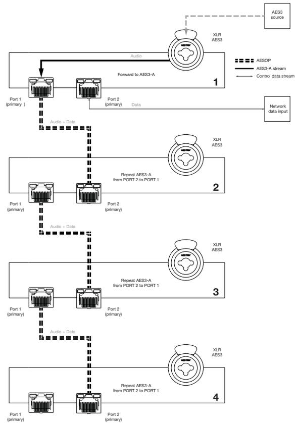
**FIGURE 41:** Daisy chain - two port models.
