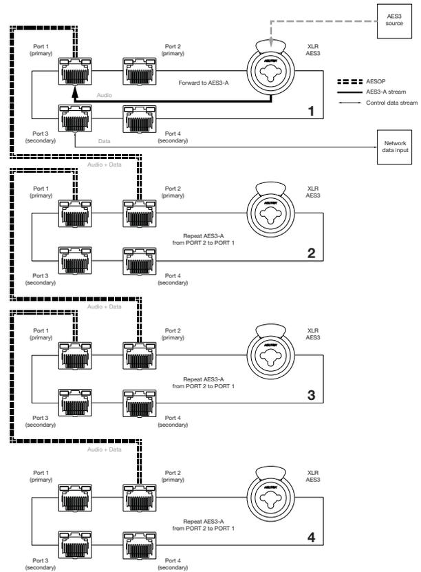
**FIGURE 40:** Daisy chain - four port models.
