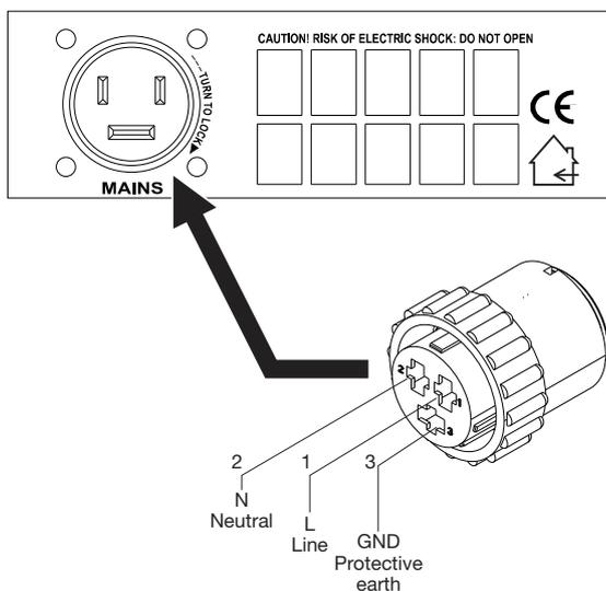
**FIGURE 7:** Mains connectors; A) IEC C20 in K2 and K3; B) AMP CPC 45A in K6, K8, K10 and K20.
