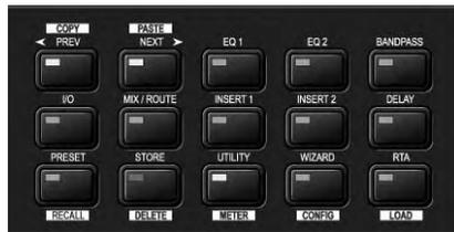
4. Now that you have reached the desired processing function, you can use the PREV or NEXT buttons to navigate through the pages of parameters available and then use the Encoder Knobs below the buttons to adjust the value.
