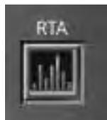
Outside of the “normal” DriveRack 4800/4820 signal path, the RTA provides an additional utility that lets you analyze incoming signals. Clicking on the RTA icon opens the RTA viewer.
