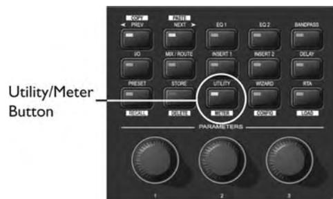
2. Scroll through the various Utility menus using Encoder Knob #1. Press the knob to enter the desired menu.
