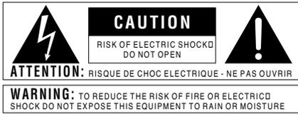
The symbols shown above are internationally accepted symbols that warn of potential hazards with electrical products. The lightning flash with arrowpoint in an equilateral triangle means that there are dangerous voltages present within the unit. The exclamation point in an equilateral triangle indicates that it is necessary for the user to refer to the owner's manual.
