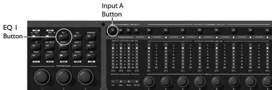
5. Edit the Graphic EQ parameters using the NEXT and PREV buttons to move between the pages. Once again, Input Channels A and B are linked so adjusting one actually adjusts them both.
