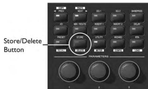
2. Select a location for this new preset in the preset table by turning Encoder Knob #1. (A preset can either be stored over an existing preset or stored in an empty location.)
