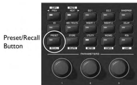
2. Press and hold the PRESET/RECALL button to enter Preset Recall mode.
