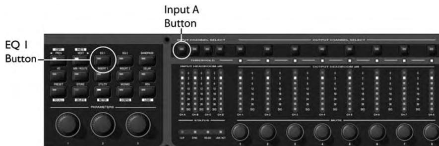
3. Turn Encoder knob #3 to link the Graphic EQs on Inputs 1 and 2.
