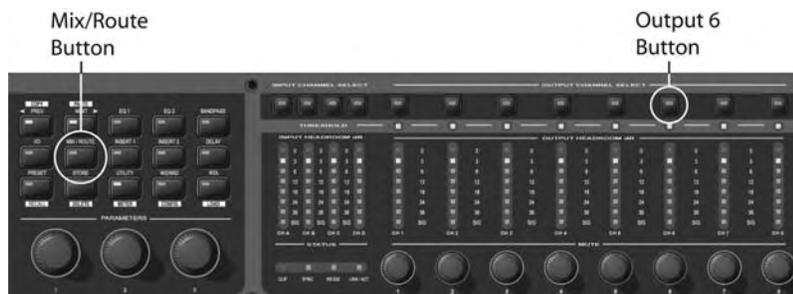
9. Make the changes by finding the Input channels A and B and adjusting their relative amounts using the Encoders.
