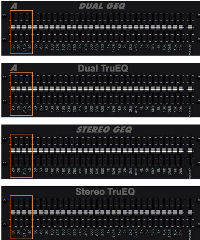
There are four standard graphic EQs that provide 31 bands of adjustment between 20 Hz and 20 kHz. A master volume slider compensates for changes in volume caused by the EQ. A maximum boost or cut of 15 dB is available for each band.
