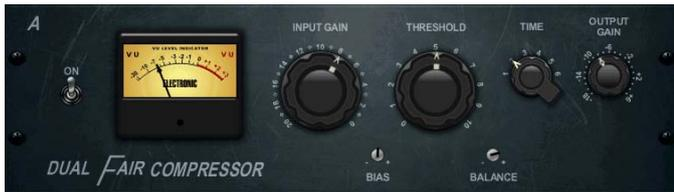
This classic tube compressor not only achieves record bids in high-end vintage gear auctions, it also delivers some of the finest colourations in compressor history. Two small trim VRs preset the control side chain action, a six-step switch determines the timing, and the two large Input and Threshold knobs adjust the levels. Our FAIR COMPRESSOR model is true to the original signal path, and conveniently provides models for dual, stereo-linked or M/S operation. *Inspired by Fairchild 670.*
