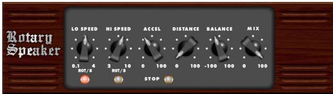
Rotary Speaker emulates the sound of a Leslie rotating speaker. The M32's Rotary Speaker provides more flexibility than its electro-mechanical counterpart, and can be used with a variety of instruments, and even vocals, to create a whirling, psychedelic effect.
