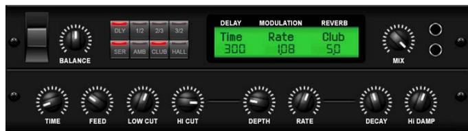
Combining echo and chorus (and in this case, reverb too) is the domain of the Modulation Delay. By combining the two, you can get the best of both worlds in one, dreamy-sounding effect.
