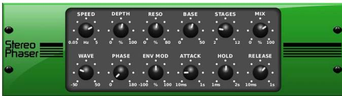
A Stereo Phaser, or phase shaper, applies multiple **STAGES** of modulated filters to the input signal to create a 'notch' in the frequency response, and then applies a **MIX** with the original for a 'swirling' effect. Use the M32's Stereo Phaser to add a 'spaced-out' sound to vocal or instrumental tracks.
