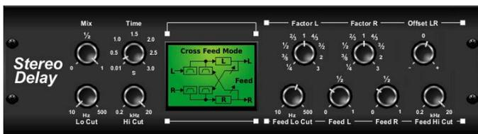
Stereo Delay provides independent control of left and right delay (echo) times, and features high- and low-pass filters for enhanced tone-shaping of the delayed signals. Use the Stereo Delay to give your mono signals a wide presence in the stereo field.
