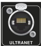
Connect to a personal monitoring system (e.g. the Behringer P16) via Ethernet cable.
