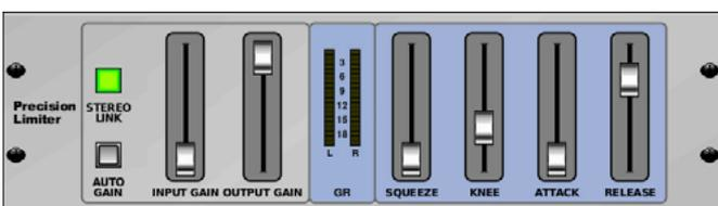
This Stereo Precision Limiter allows you to set a precise volume limit, ensuring distortion-free, optimal signal integrity. Use the M32's Stereo Precision Limiter to boost quiet signals or prevent clipping while preserving the level of ‘hot’ signals.
