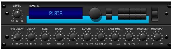
A plate reverb was originally created by sending a signal through a transducer to create vibrations on a plate of sheet metal which were then picked up as an audio signal. Our algorithm simulates that sound with high initial diffusion and a bright-coloured sound. The M32's Plate Reverb will give your tracks the sound heard on countless hit records since the late 1950s. *Inspired by the Lexicon PCM-70.*
