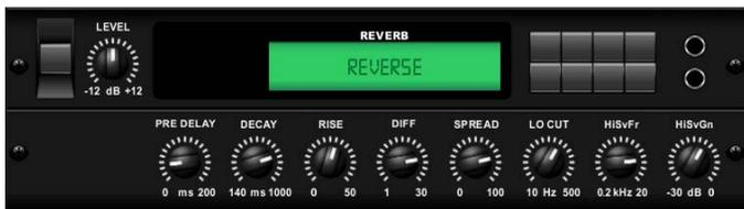
Reverse Reverb takes the trail of a reverb, turns it around, and places it in front of the sound source. Use the swelling crescendo of the Reverse Reverb to add an ethereal quality to vocal and snare drum tracks. *Inspired by the Lexicon 300/480L.*
