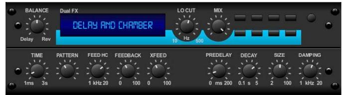
Here we have combined Delay and Chamber reverb, so that a single device can supply a variety of delay settings, plus add just the right amount of reverb to the selected signal. This device only uses one effects slot. *Inspired by the Lexicon PCM 70.*
