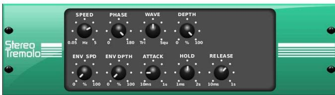
Stereo Tremolo creates an up and down volume change at a constant and even tempo just like the guitar amps of yesteryear. Use the M32's Stereo Tremolo to add a unique 'surf-music' texture to a vocal or instrumental track.
