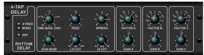
The Rhythm Delay, or 4-Tap Delay, provides four delay stages with independent frequency, gain and pan controls. Create time-based echo effects with the triple delay to increase the sense of stereo separation.
