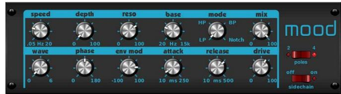
The Mood Filter uses an LFO generator and an auto-envelope generator to control a VCF (voltage-control filter), as well as a side-chain function, where the channel B signal controls the envelope of channel A. When applied to electronic instruments, the Mood Filter can be used to emulate the natural sound of acoustic instruments. *Inspired by the MiniMoog.*
