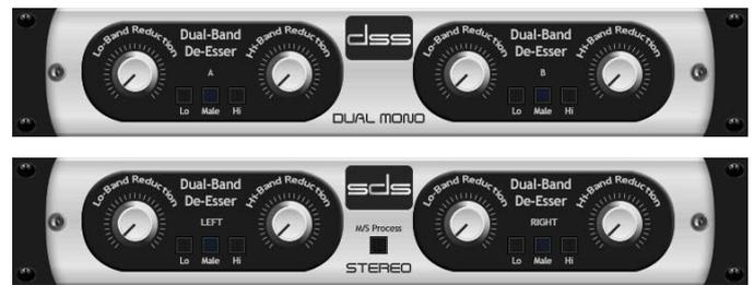
De-essing is an audio effect designed to reduce the amount of excessive sibilance in an audio signal, usually when dealing with the human voice. The Dual DeEsser accurately and seamlessly removes sibilance from audio tracks.
