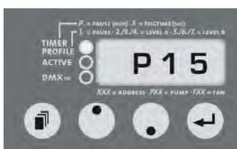
Fig. 5: Adjusting the performance of the fog generator
